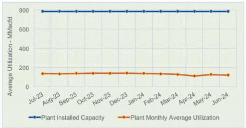
Figure 7: TPDC pipeline capacity utilization
